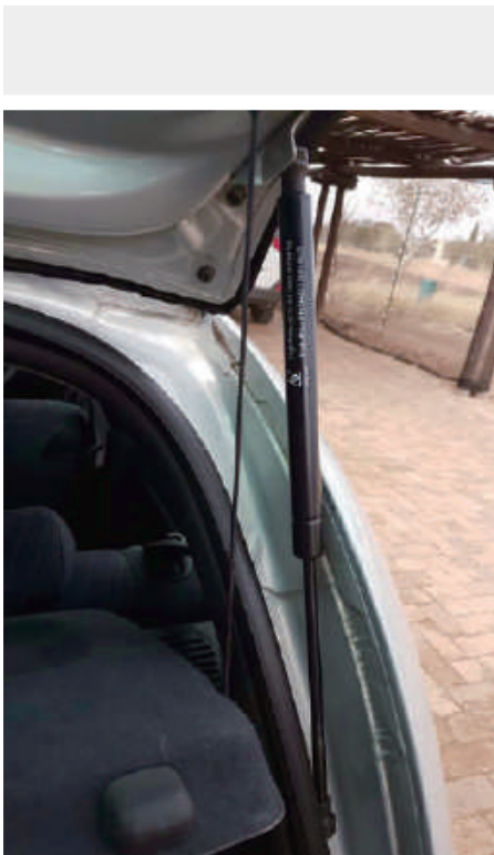
20-Plastic ball with brackets gas spring Plastic ends can be used with a variety of brackets
